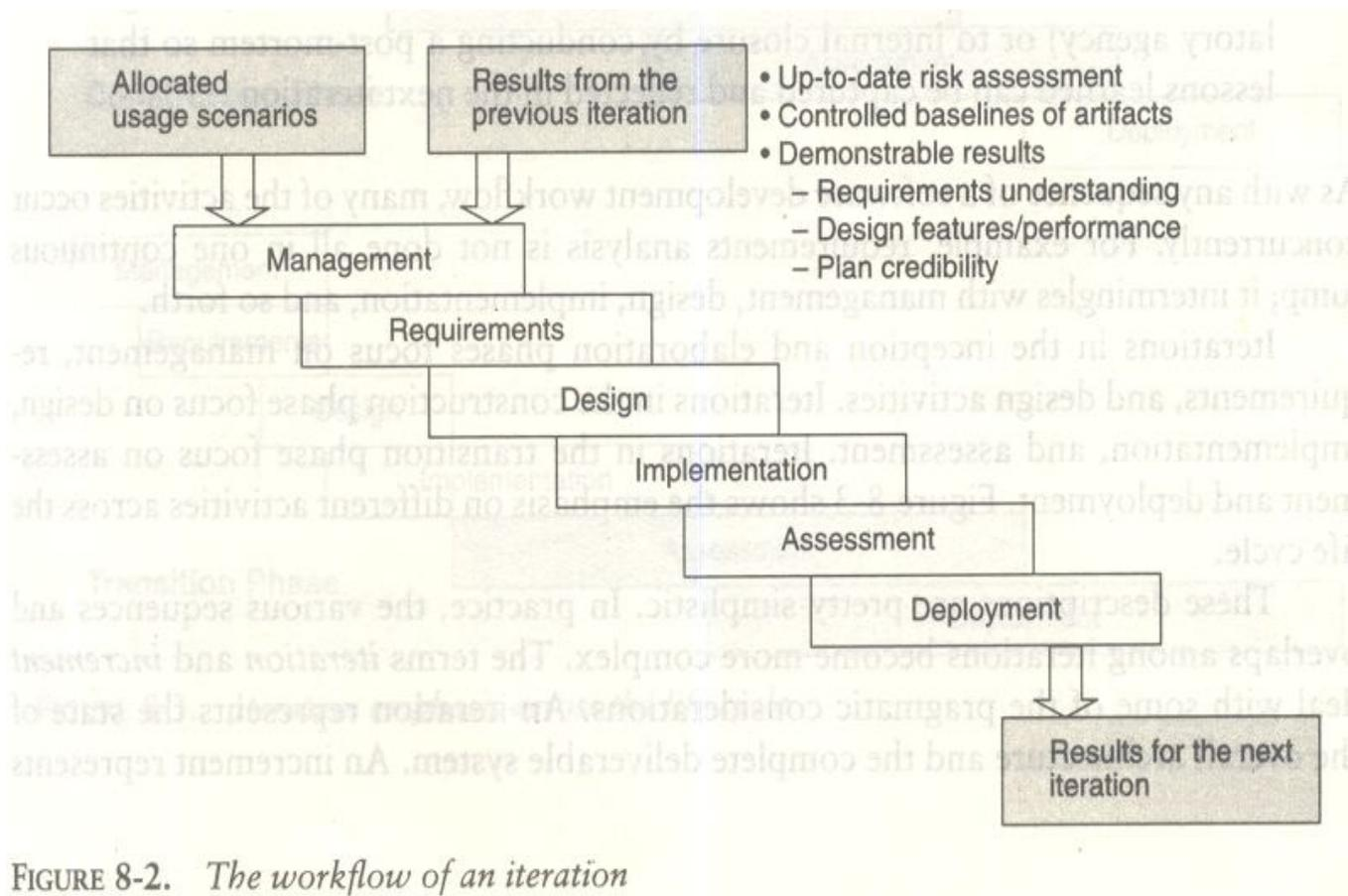
FIGURE 8-2. *The workflow of an iteration*
